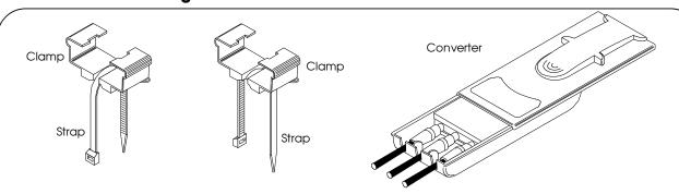
Make connections between LNB and Converter with supplied 90 cm. F / F coaxial cables.
