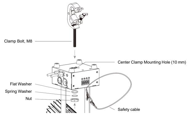
To clamp the fixture to a truss:
