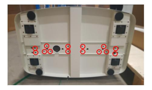
**Step 5**Begin screwing the bolts clockwise into each of the holes using an **Allen Wrench** to secure the two pieces together.
