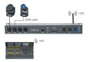
Notes: 1). connect your lighting console to the Recorder's WiFi hotspot (password: 12345678). 2). Set IP address of your lighting console in the same network range as Recorder's WiFi IP address (2.0.0.x). 3). ArtNet output from your console must be enabled.
