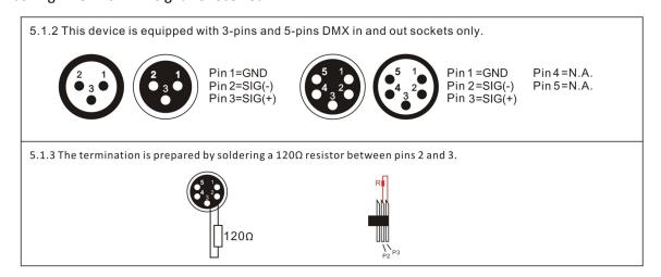
5.1.4 Connection: us DMX cable with 3+5-pin XLR-plugs to connect the controller with the fixture or one fixture with another.
