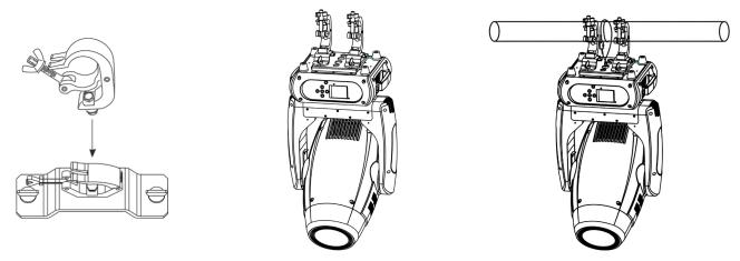
Step one: Installation the clamp onto the omega bracket;
