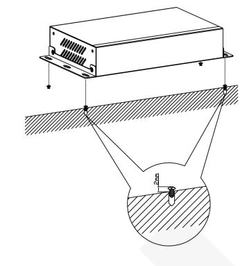
Step 1: Install the SWT screws on a platform, and leave a 2mm high clearance.
