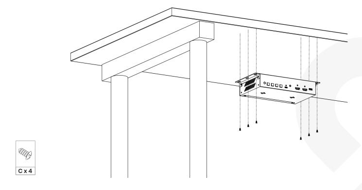
Step2 - Use 4 SWT screws to firmly fix HUS03-4K6G beneath the table.
