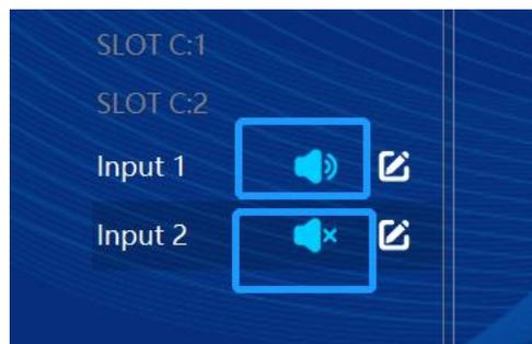
There is only one input signal can be enabled with audio and routed to the 3.5mm output at the rear panel of iWall X. When turn on audio for one input signal, the other audio channels from other inputs will be muted automatically.
